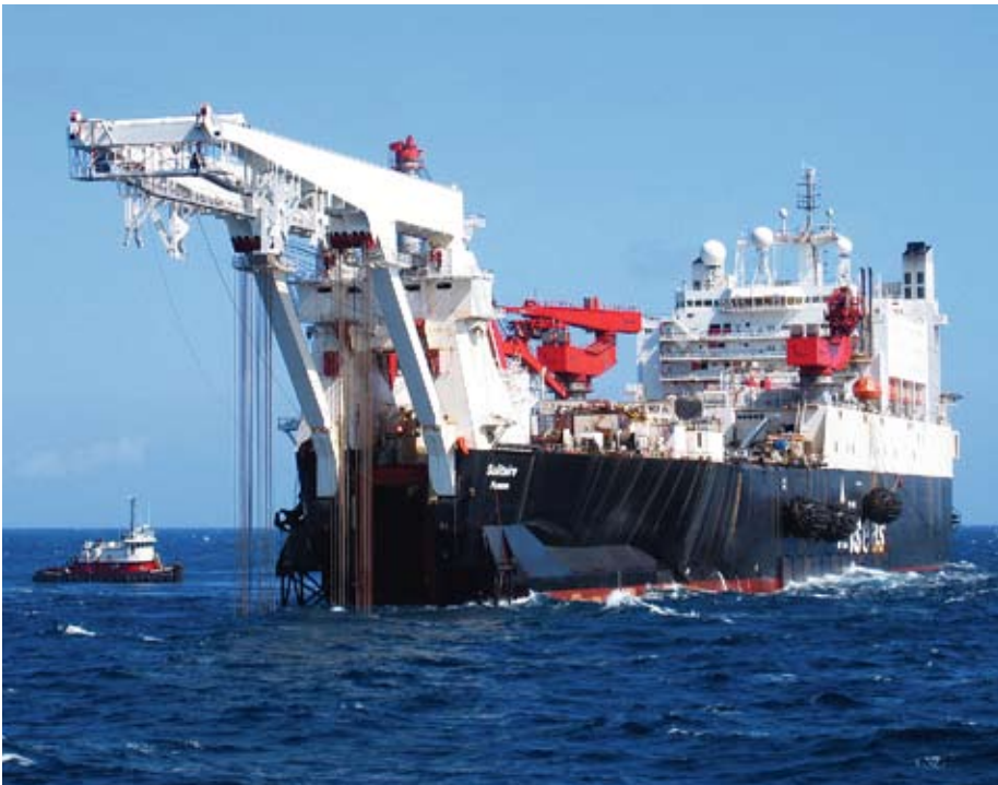
Allseas' Solitaire is the largest pipelay vessel in the world. It is one of three vessels involved in the construction of the Nord Stream pipeline.
